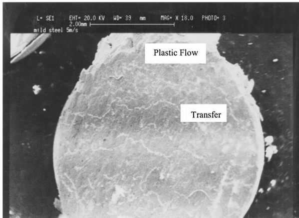
Figure 8 Scanning electron micrograph of the MS pin surface tested at a sliding speed of 5 m/s.
